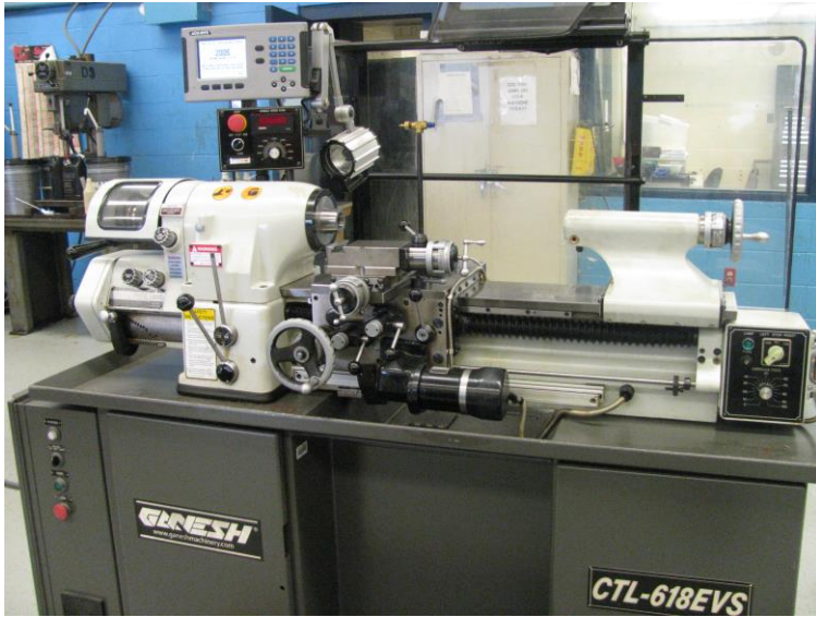
Ganesh Tool Room lathe Similar to the machine above the Ganesh Lathes are great for small precision work.
